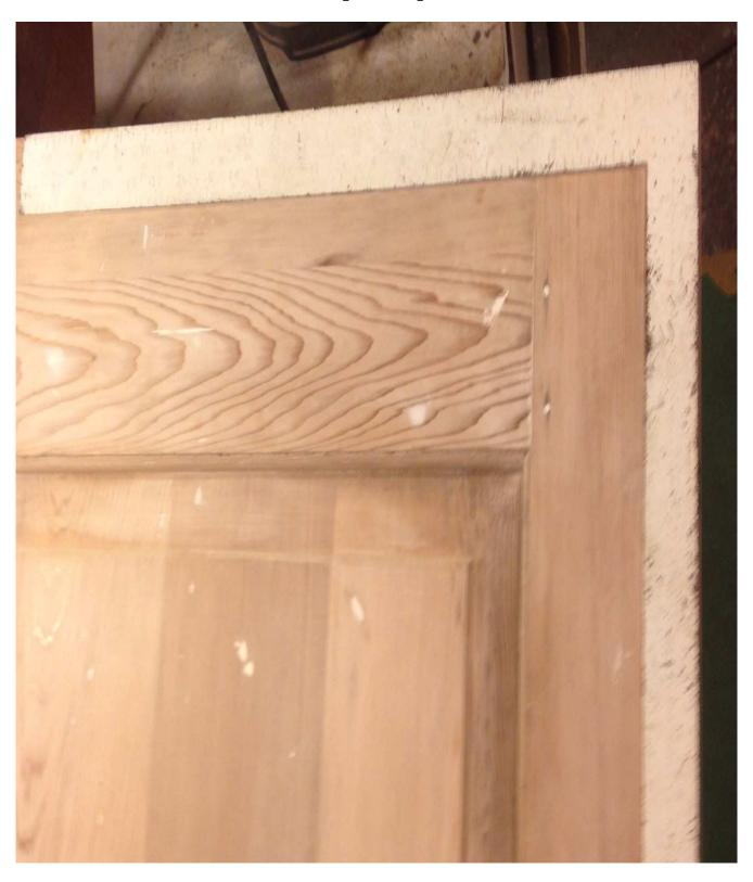
Keeping in mind that this is a cottage door, the next step is to make sure that the sides are square. In my design, I elected to have the door knob hole at the bottom so that it would lie below the mattress and bed covers. Use a carpenter's square to determine if both ends are square. In my case, the bottom of the
