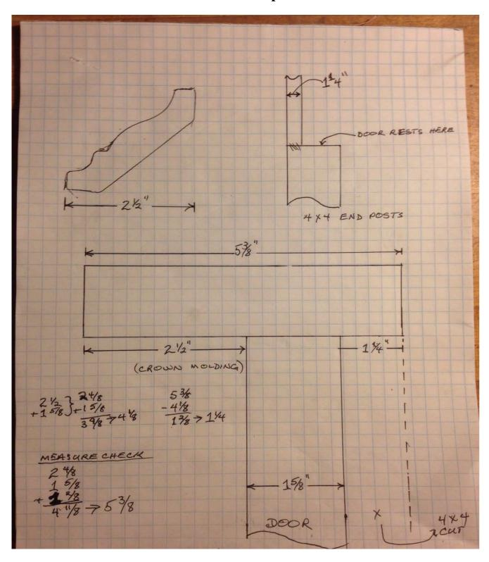
The crown molding I chose is the starting point. The plan shows that its installed depth is two and one-half inches (2.5"). This is used to determine where the top board will be positioned on the hinge-side of the door as well as the amount of overhang on each side of the door thus giving you the actual length of
